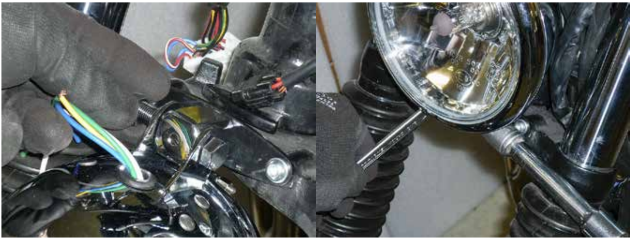
Apply and fasten headlamp.
