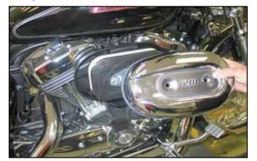
2. Remove the two air filter cover mounting bolts and then remove the cover from the vehicle as
