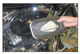
4. Remove the air filter as shown.
