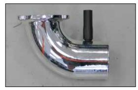
9. Cut the provided crankcase vent hose to a length of 1.75" and install onto the K&N $^{\odot}$  intake tube as shown.
