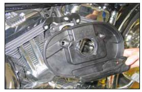
6. Remove the air filter base as shown. NOTE: K&N Engineering, Inc. recommends that customers do not discard the factory air intake components. 8. Install the K&N<sup>®</sup> intake tube adapter onto the throttle body using the provided hardware. NOTE: Apply one drop of the provided thread locker to the three tube adapter mounting bolts.
