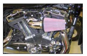
11. Install the K&N<sup>®</sup> air filter onto the K&N<sup>®</sup> intake tube and secure with the provided hose clamp. A black hose clamp is being supplied with kit. This clamp is intended to clamp the filter to the intake tube.
