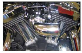
10. Install the K&N<sup>®</sup> intake tube onto the throttle body while attaching the vent hose to the vent tube and secure with the provided hardware. **NOTE: Apply one drop of the provided thread** locker to the K&N<sup>®</sup> intake tube mounting bolts, adjust the vent tube and intake tube/throttle body for best fit, and tighten the mounting bolts.
