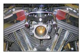
7. Install the K&N<sup>®</sup> crankcase breather tube onto the vehicle using the provided hardware. **NOTE: Do not completely tighten the breather bolts at this time.**
